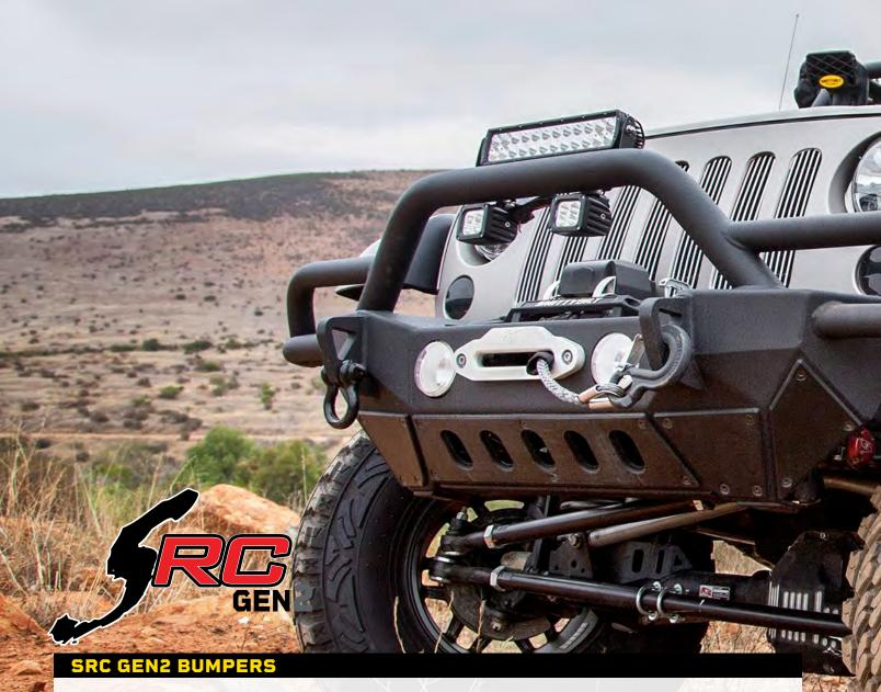
The SRC Gen2 bumpers have been completely redesigned for greater fender-to-fender protection. Manufactured from 3/16" cold rolled steel, the bumpers feature corners that extend to match the factory fender lines. The raised corners allow for better entry and exit angles in extreme conditions.
