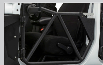
G 1.5" diameter 090 wall steel tubing
