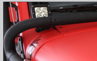
B 1.75" diameter 0.120-wall steel tubing
