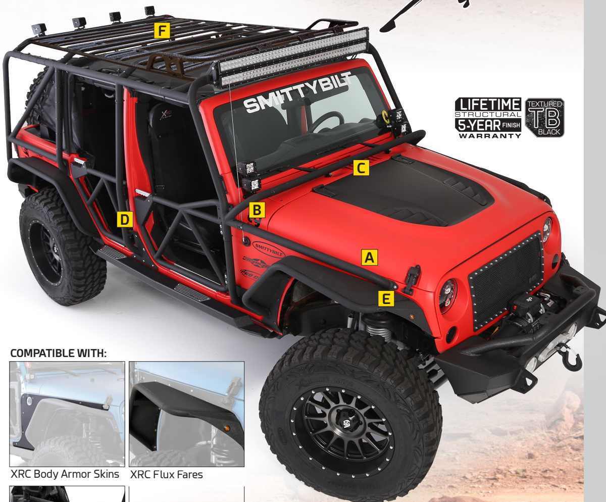
C Windshield crossbar for roof access
