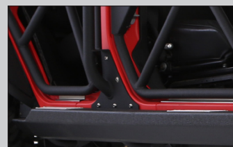
D B-pillar fixing point to reduce swaying
