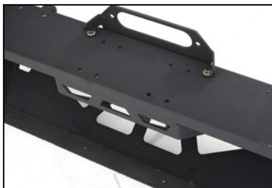
Integrated winch plate for up to 12,000 lbs
