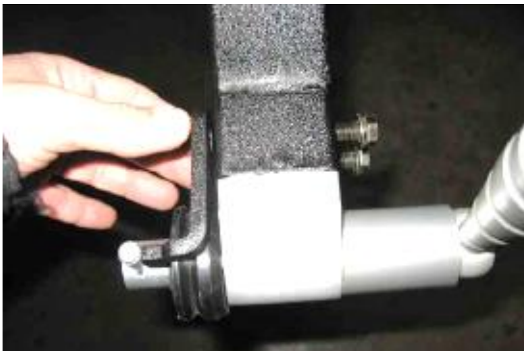
76856-06 Latch support bracket install.
