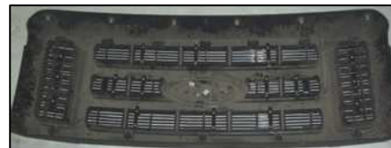
Figure 7 – Rear view of vehicle's shell; Billet Grills attached with Metal Brackets and Flange Nuts
