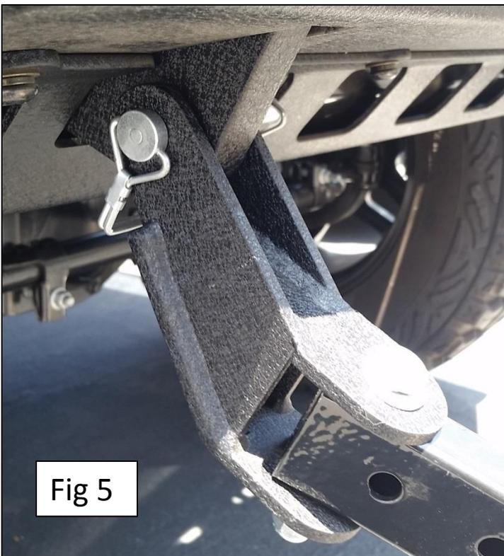
Step 7. Center tow bar and brackets on vehicle, then tighten all hardware. Check torque on all hardware and inspect tow bar before each used.
