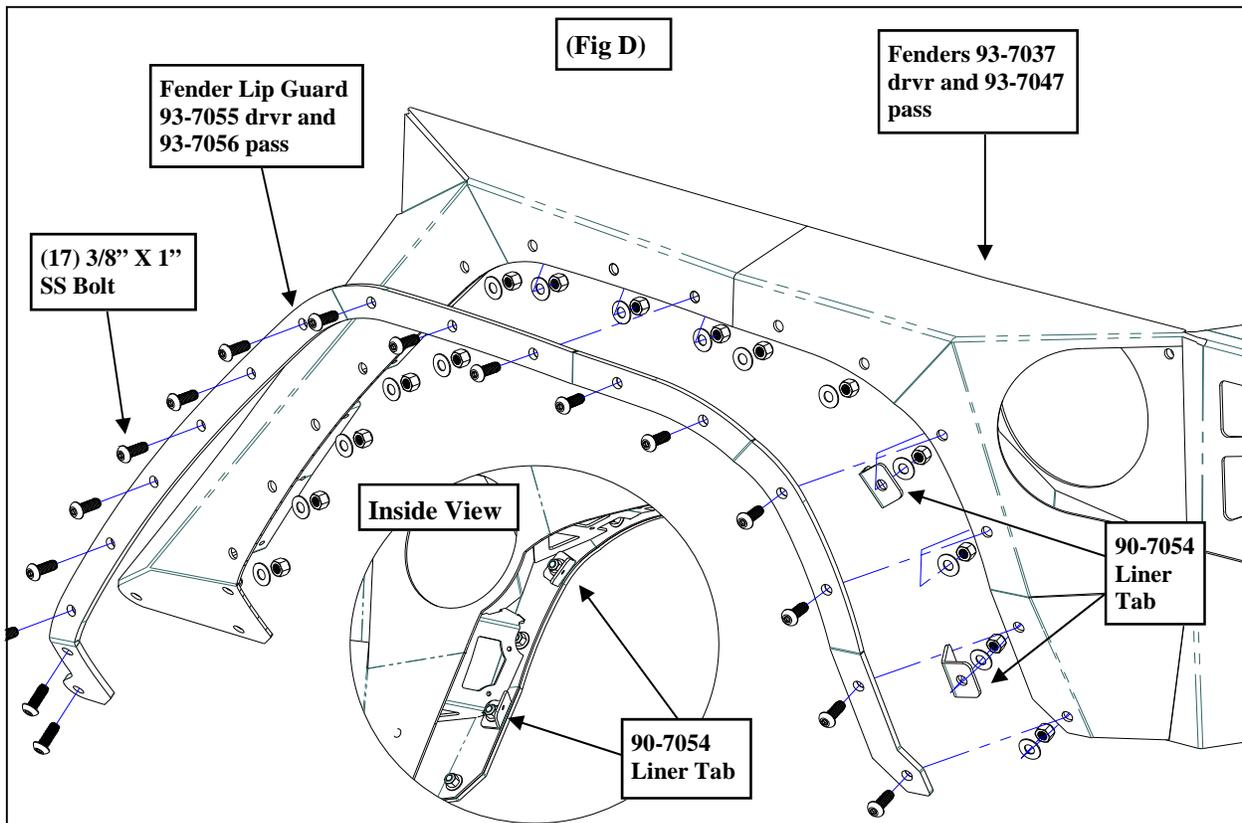
**Step 13:** Remove the clamps and secure the armor fender using the supplied 3/8" X 1" bolts and hardware. Be sure to start all the bolts by hand to avoid cross threading the bolts. Fig. B & C.
